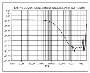
Note: Spikes at high frequencies are induced by the PCB layout
